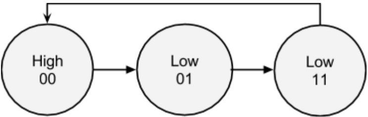
Gray coding (with violation from state 11 to state 00) (Fig. 29)
